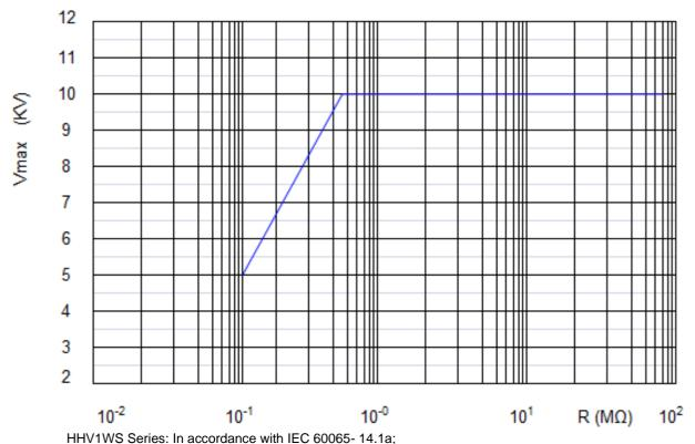
50 discharges from a 1 nF capacitor charged to Umax; 12 discharges/min
