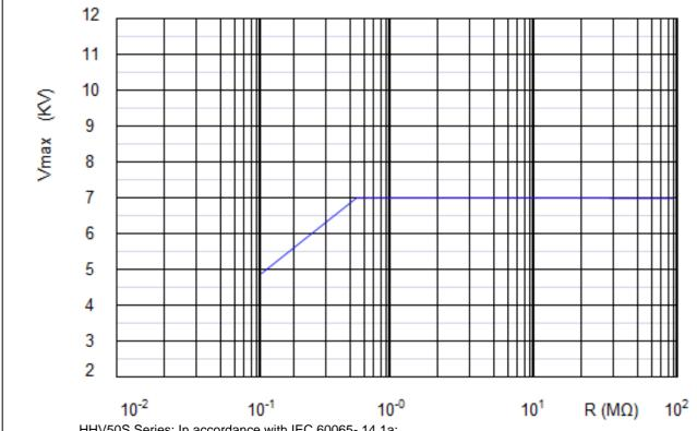
HHV50S Series: In accordance with IEC 60065- 14.1a; 50 discharges from a 1 nF capacitor charged to Umax; 12 discharges/min
